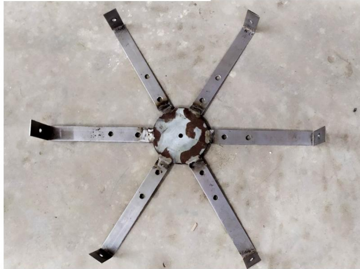
Fig. 4.4: Weld all 6 L-clamps on the plate washer
