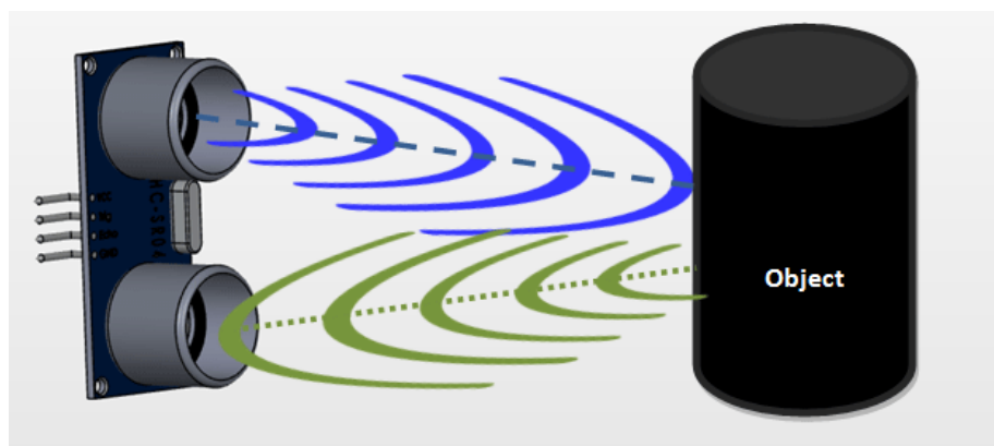
Figure 3.9: Ultrasonic Sensor detecting an object
