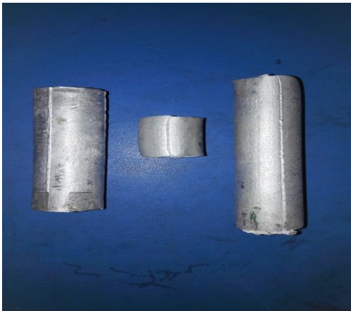
(c) Double shear strength test sample of Al+JSA
