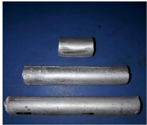
(b) Double shear strength test sample of Al+CDA
