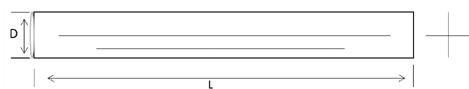
Fig 7: Double shear strength test specimen
