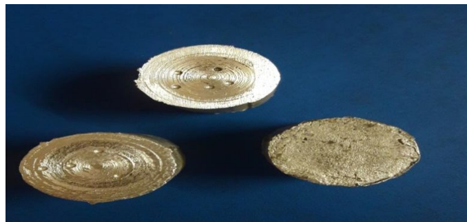
(b) Hardness Test Sample of Al-JSA and Al+RHA+CDA+JSA
