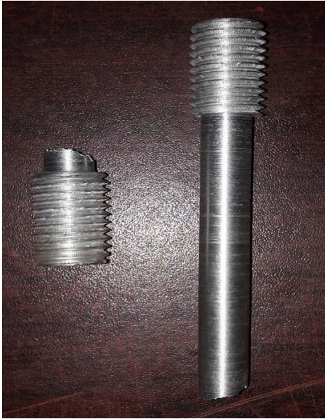
(a) Tensile test sample of Al+RHA
