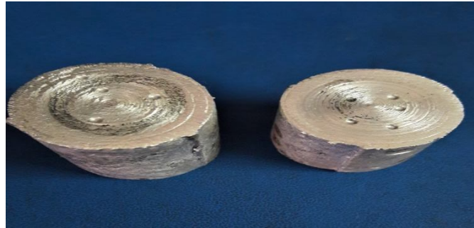
(a) Hardness test sample of Al-RHA and Al-CDA
