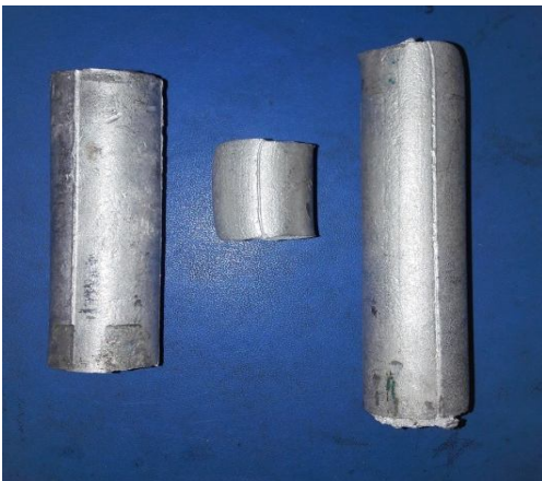
(a) Double shear strength test sample of Al+RHA
