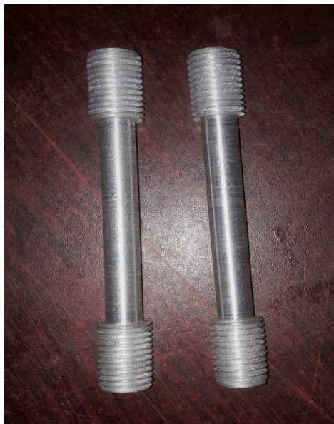
(c) Tensile test Sample of Al+JSA
