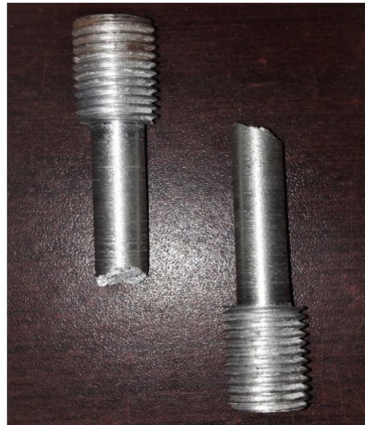
(b) Tensile test sample of Al+CDA
