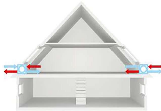
Mechanical ventilation: Balanced decentral supply and extract
