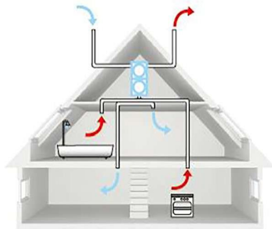
Mechanical ventilation: Balanced central supply and extract
