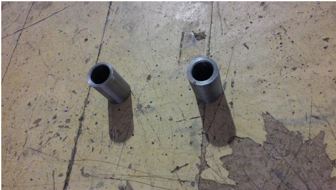
Fig. 5.4: Trunnions with internal threading
