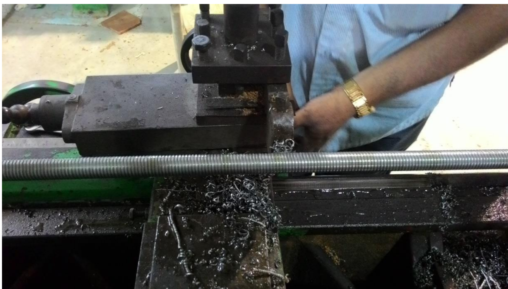
Fig. 5.2: Fabrication of power screw on lathe
