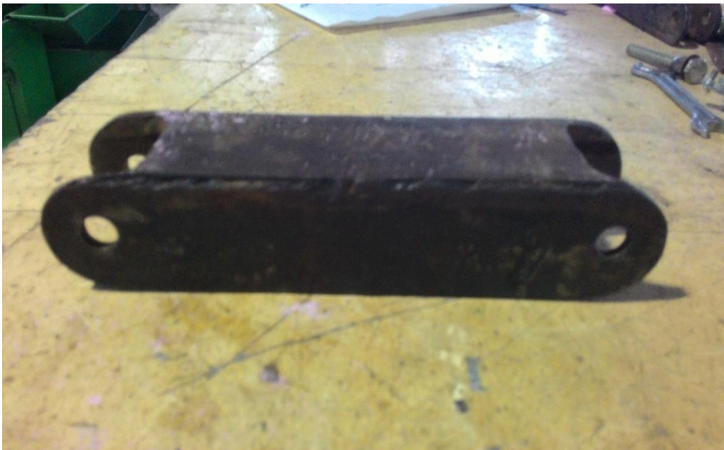
Fig. 5.3: Arm of Scissor Jack
