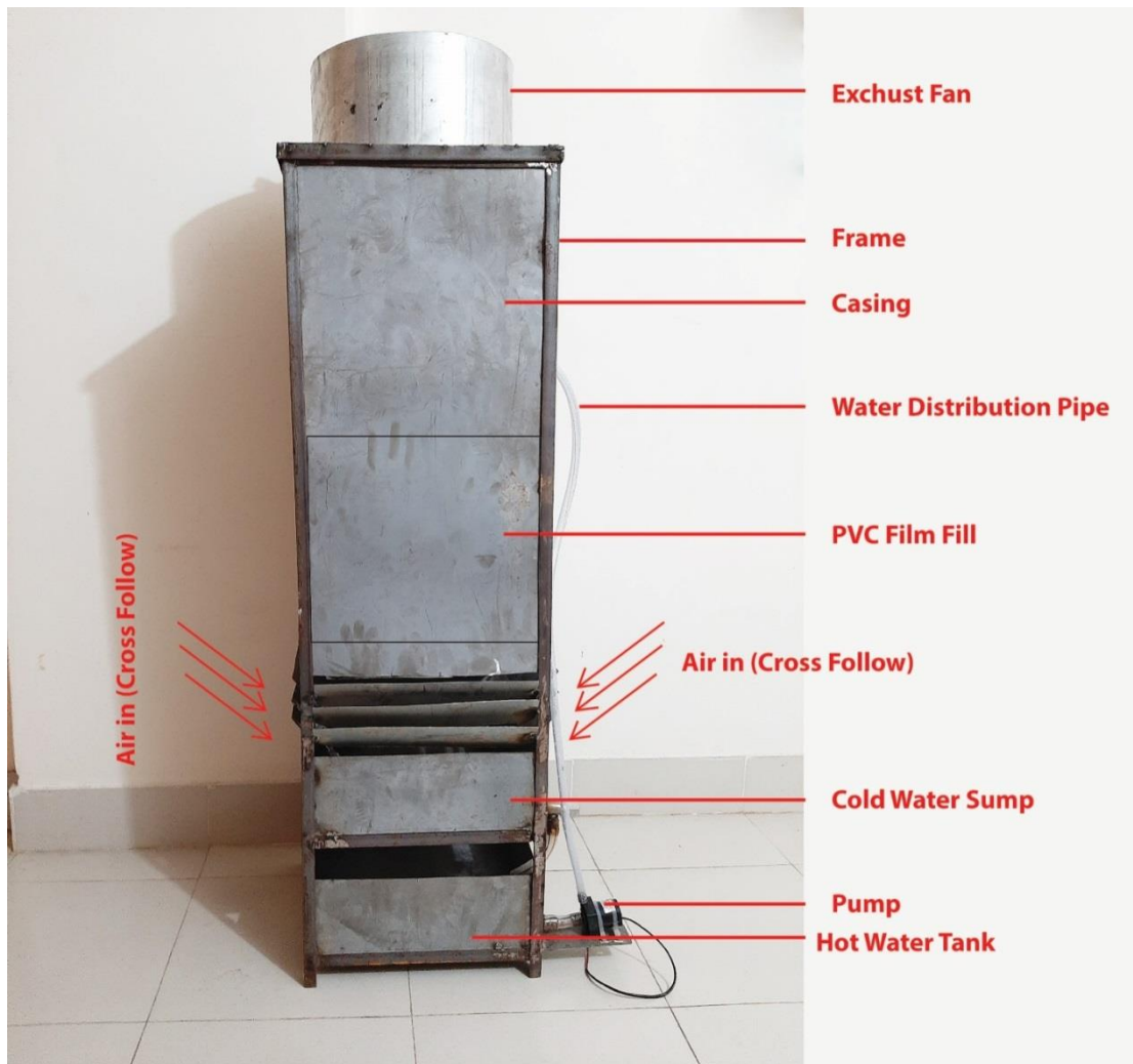
Fig. 4.1: Induced draft counter flow cooling tower
