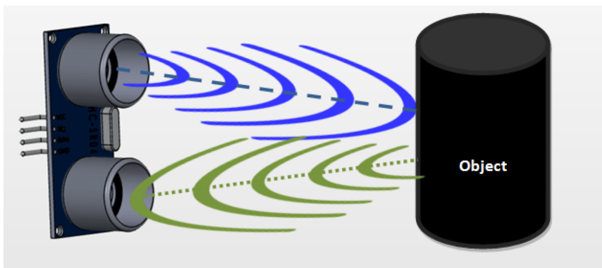
Figure 2.20: Ultrasonic Sensor Working Procedure
