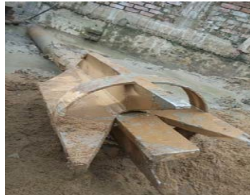
Fig: 3.4. Drilling bit/chisel for piling
