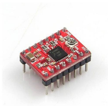
Figure (3.4); Stepper motor Drivers with heat sink
