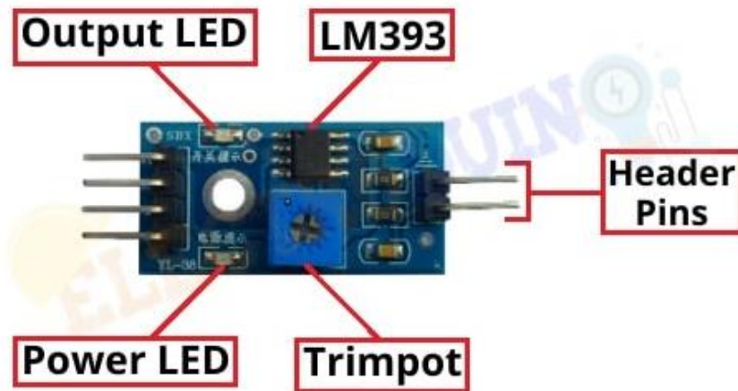
Figure 3.11: Rain Sensor Pin Indication & Description
