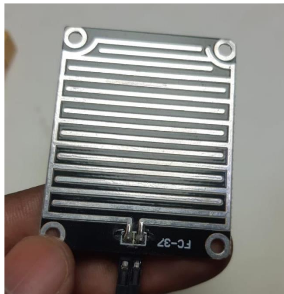
Figure 3.10: Rain Sensor Pin Diagram
