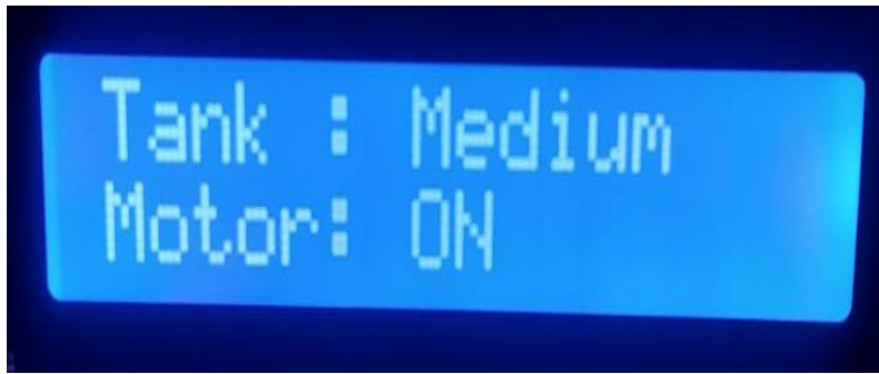
Fig 4.2: Medium Tank Alarm
