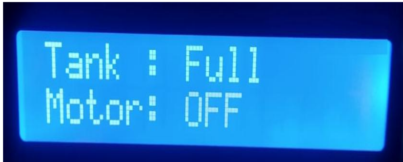
Fig 4.3: Tank Full Alarm
