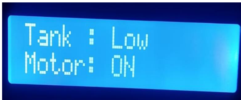
Fig 4.1: Low Tank Alarm
