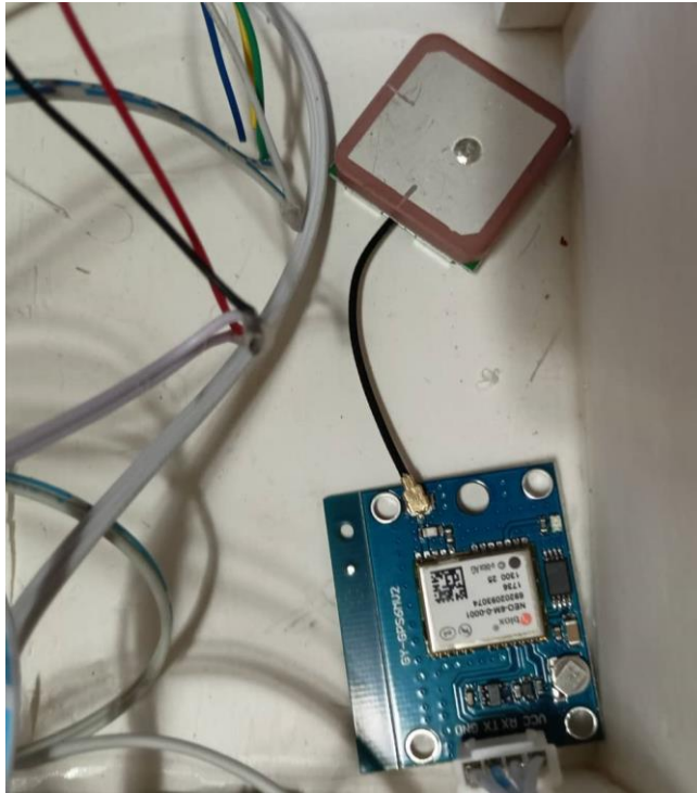
Fig 3.10: GPS Setup at Vehicle
