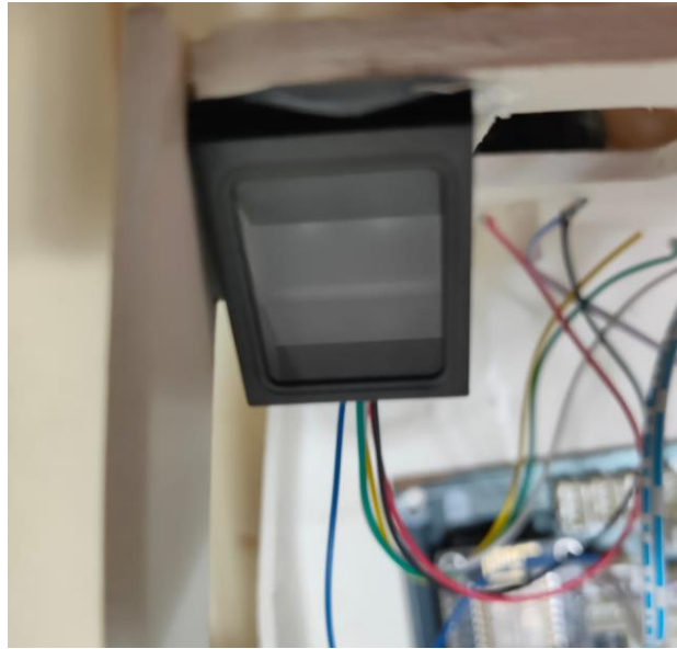
Fig 3.3: Finger Print Sensor attached in vehicle
