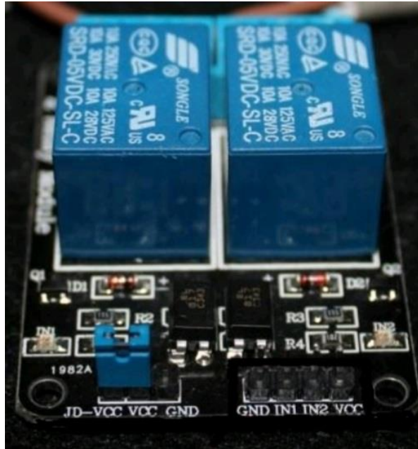
Figure 3.10: Main Voltage Connection
