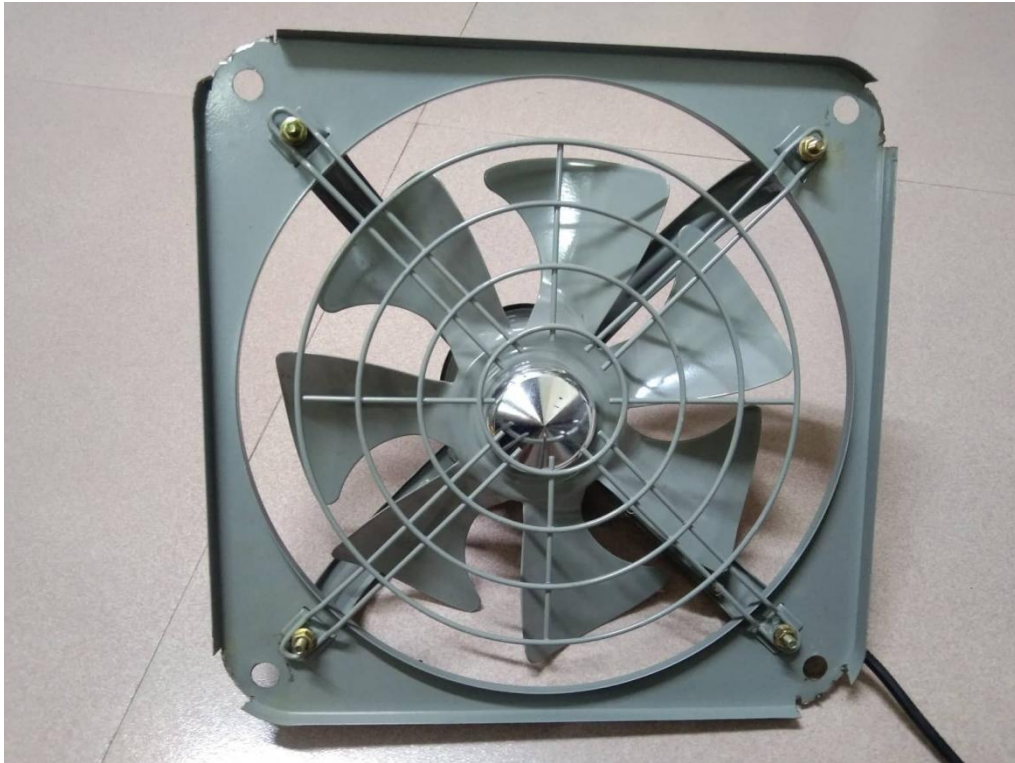
Figure 3.3: Industrial Exhaust Fan (Front Side)
