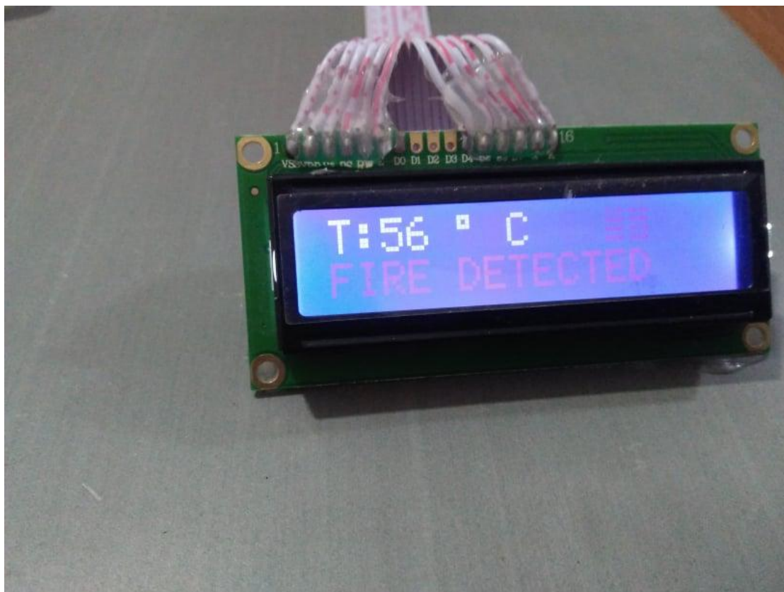
Figure 6. 2 Testing fire near the temperature sensor.
