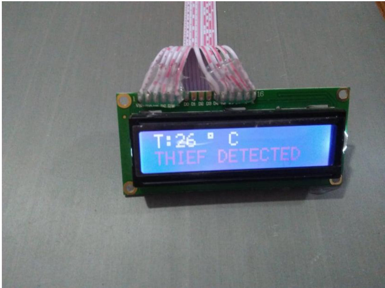
Figure 6. 3 Testing the PIR sensor for detecting intruder. (b) Thief detection mobile notification. (c) LCD display showing thief detected.
