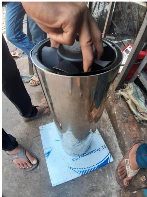
Figure 4.5: Exhaust Fan setup on Air Cylinder Structure
