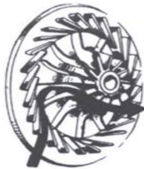
FIG: 6.17 AIRFLOW THROUGH A RADIAL-INFLOW TURBINE
