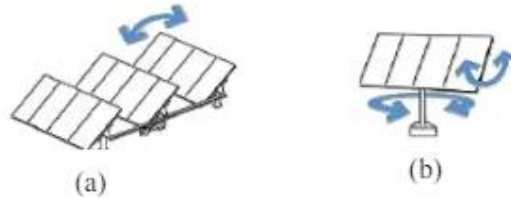
Figure 2.17: (a) Schematic diagram of single axis solar tracker (b) Schematic diagram of double axis solar tracker
