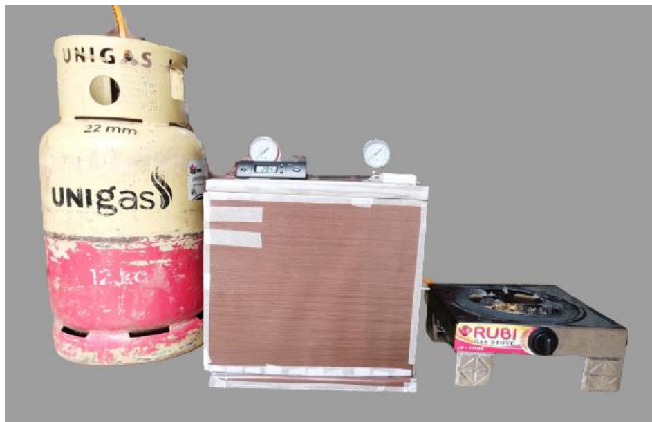
Figure. 15. LPG refrigeration and heating system
