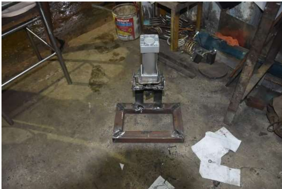
Figure 4.6: After Setup pneumatic cylinder with hardware
