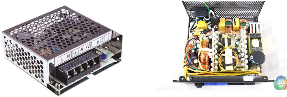
Figure 4.13 SMPS (Switch Mode Power Supply)
