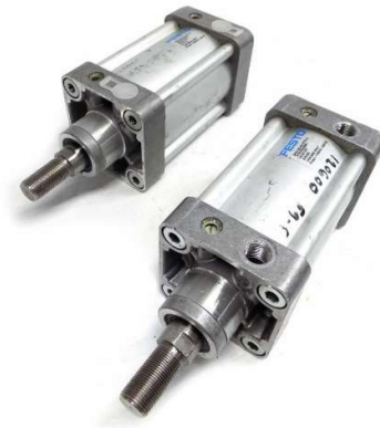
Figure 4.17: Pneumatic Air Cylinder
