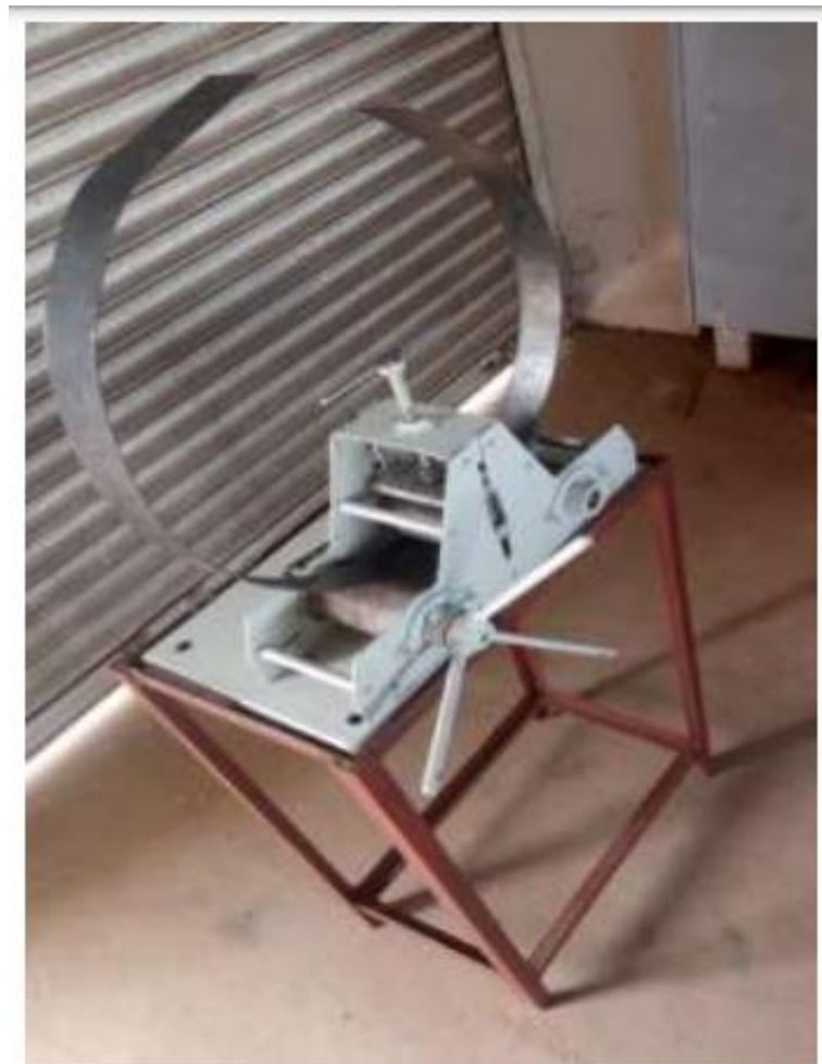
Figure 2.2: Manual Roller Bending Machine (Pachange, 2019)
