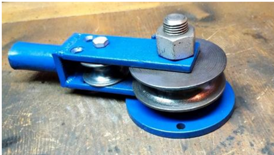
Figure 3.8: Pipe Bending Handle Mechanism
