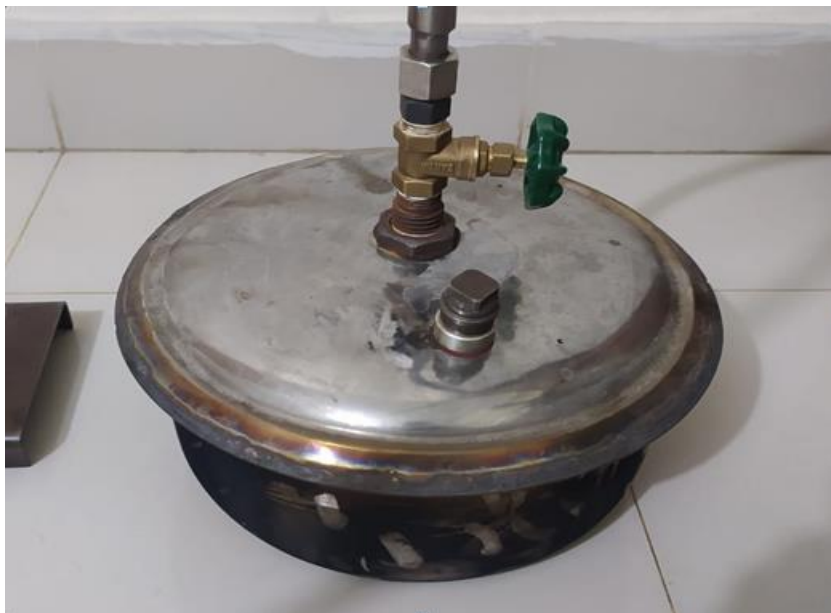
Figure3.3: Boiler of steam engine
