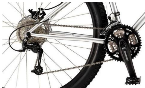
Figure 4.7: Multi-speed gear system
