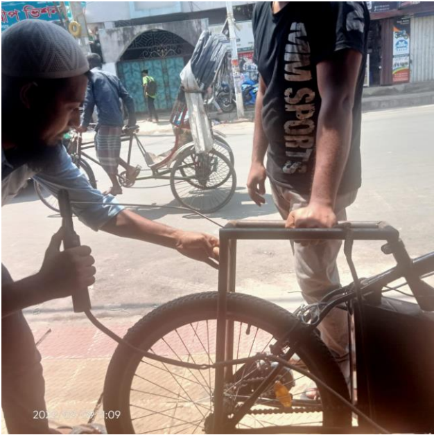
Figure A.1: Welding the customized seat
