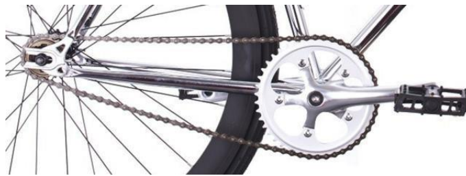
Figure 4.6: Fixed gear system
