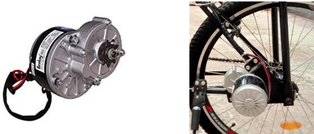
Figure 4.1: PMDC Side Motor
