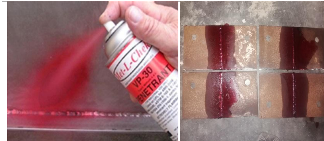
Fig-4.2: Application of penetrant
