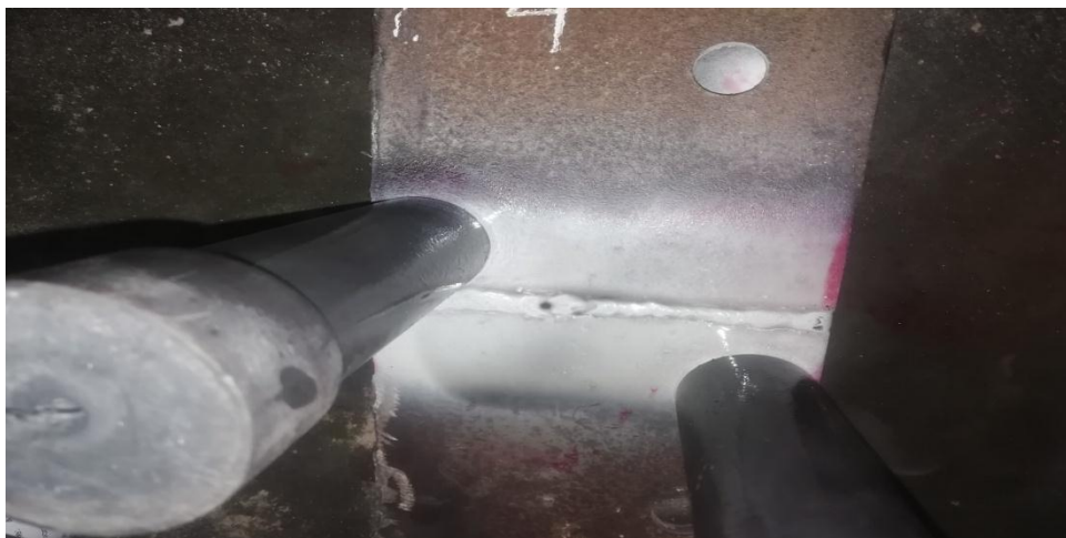
Fig-5.5: Penetration of Magnetic Flux
