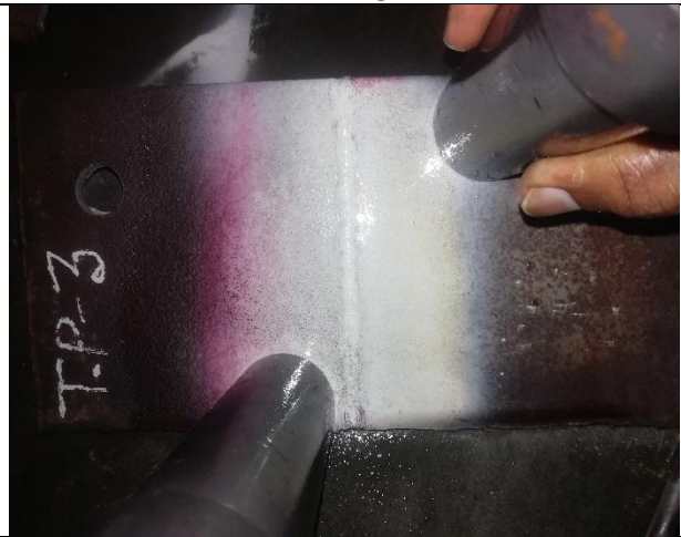
MPI of Welding Plate-3
