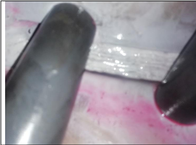
MPI of Welding Plate
