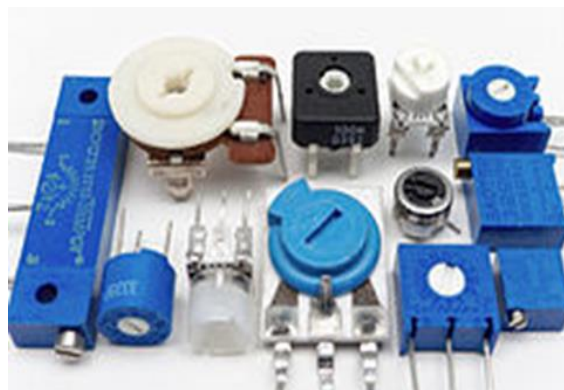
Fig: 2.2.13.2: Different Types of Potentiometer
