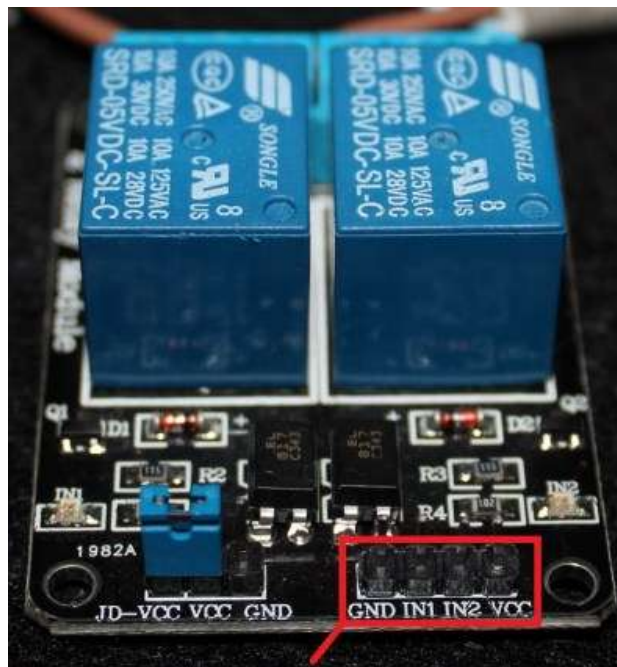
Figure 3.15: Main Voltage Connection
