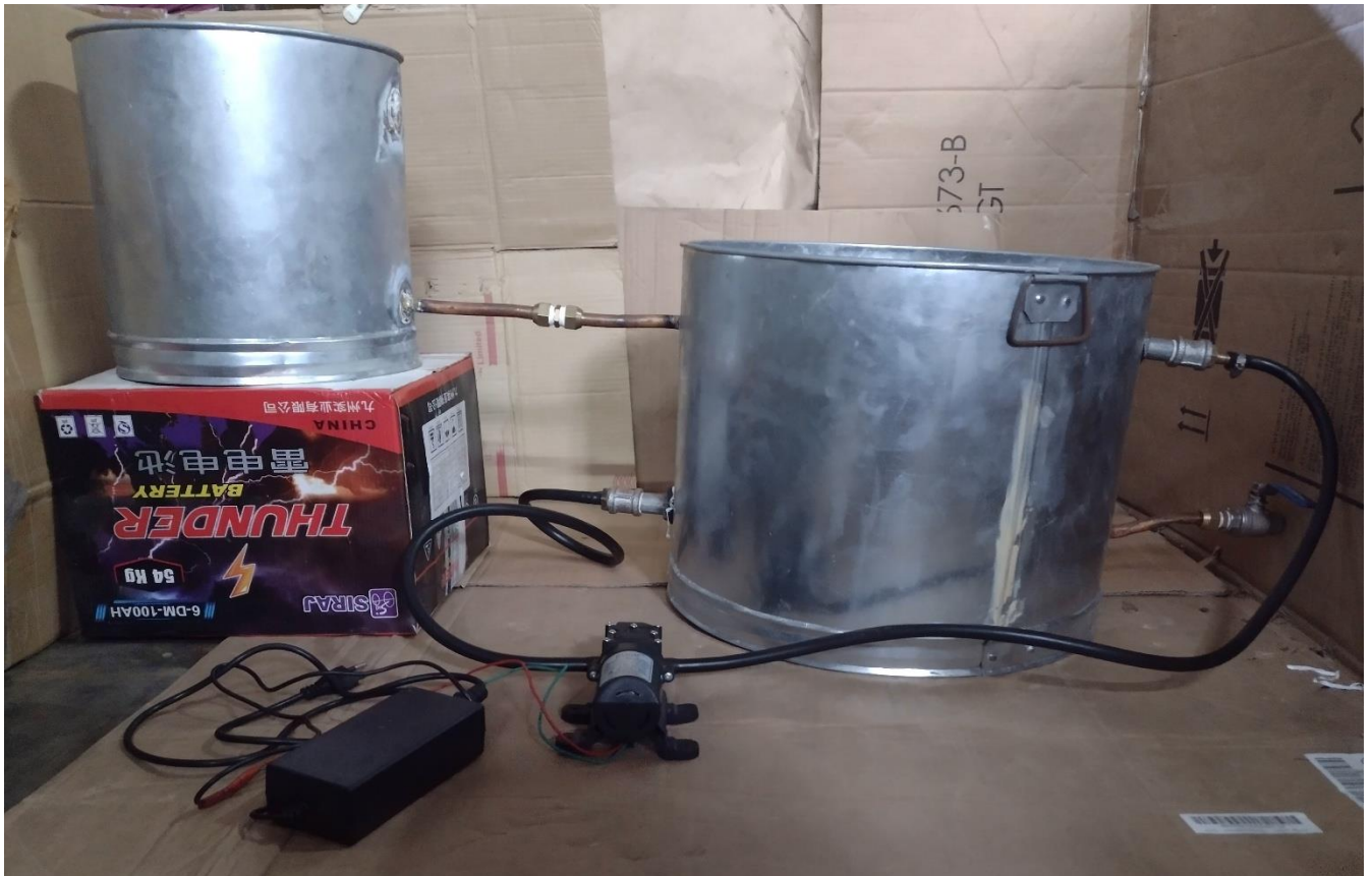
Figure 3.17: Experimental Setup of Helical Tube Heat exchanger
