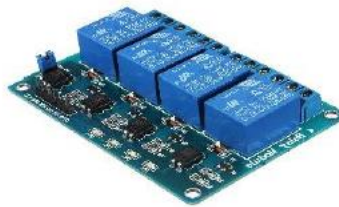
Fig 3.5: A 5v 4 channel relay module
