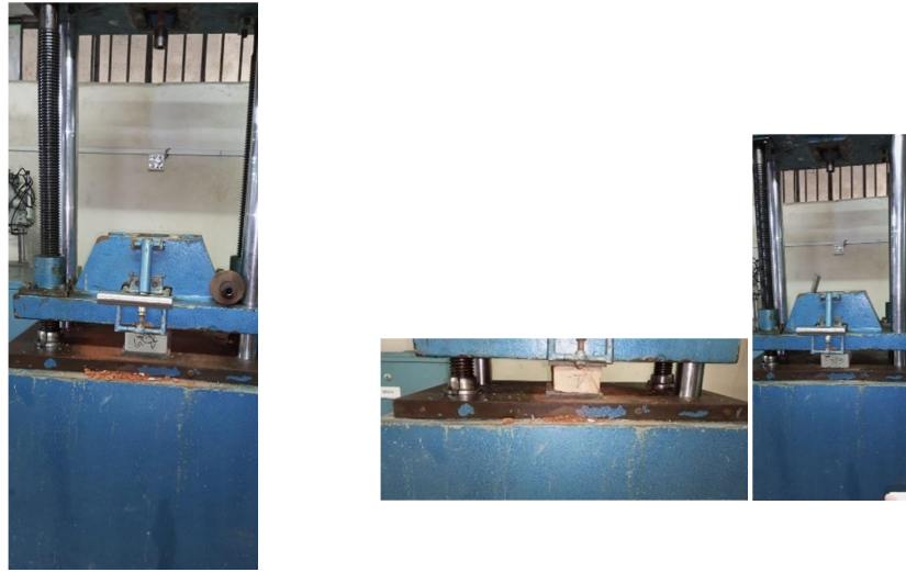
Figure 3.1.2: Typical setup for compressive strength determination
