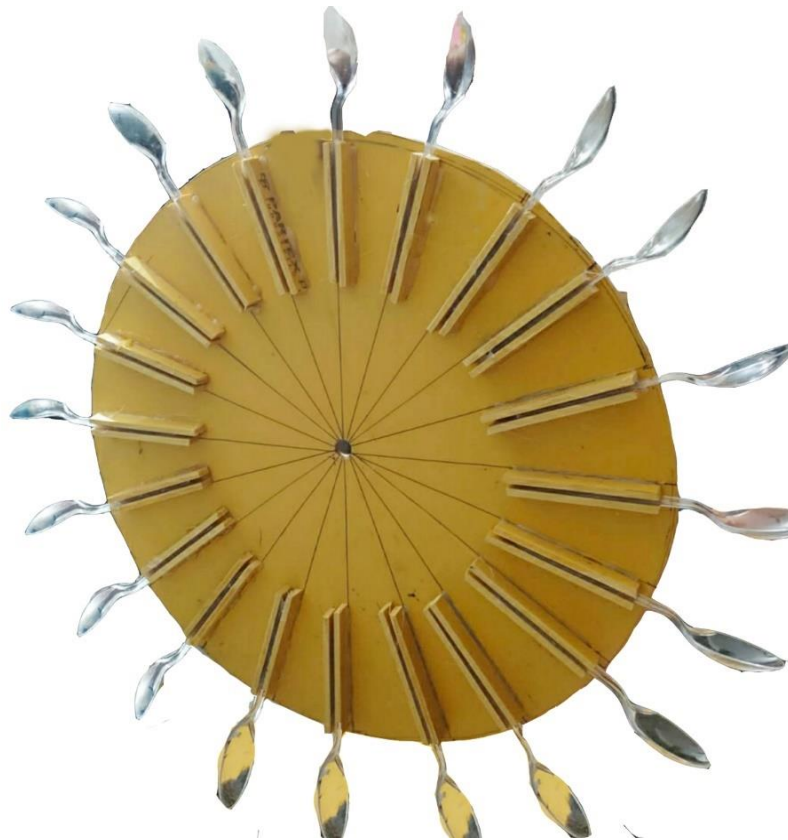
Figure 4.10 construction of water turbine
