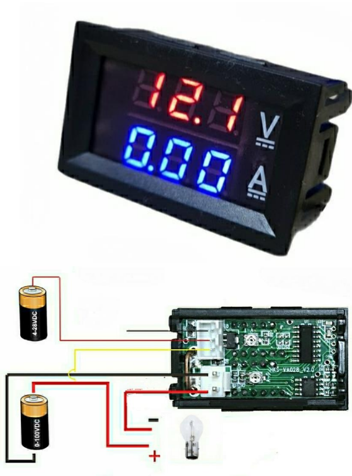
Figure 4.6 Voltmeter & Ampere meter
