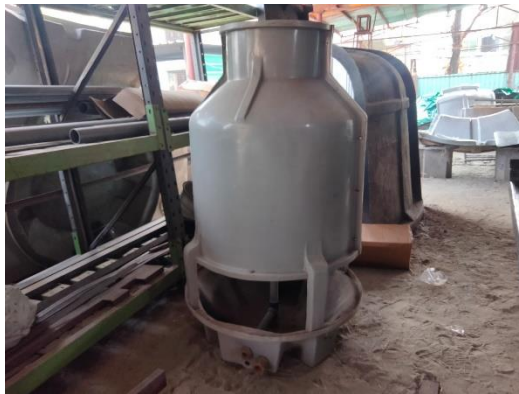
Fig 3.3: Bottled induced draft cooling tower
