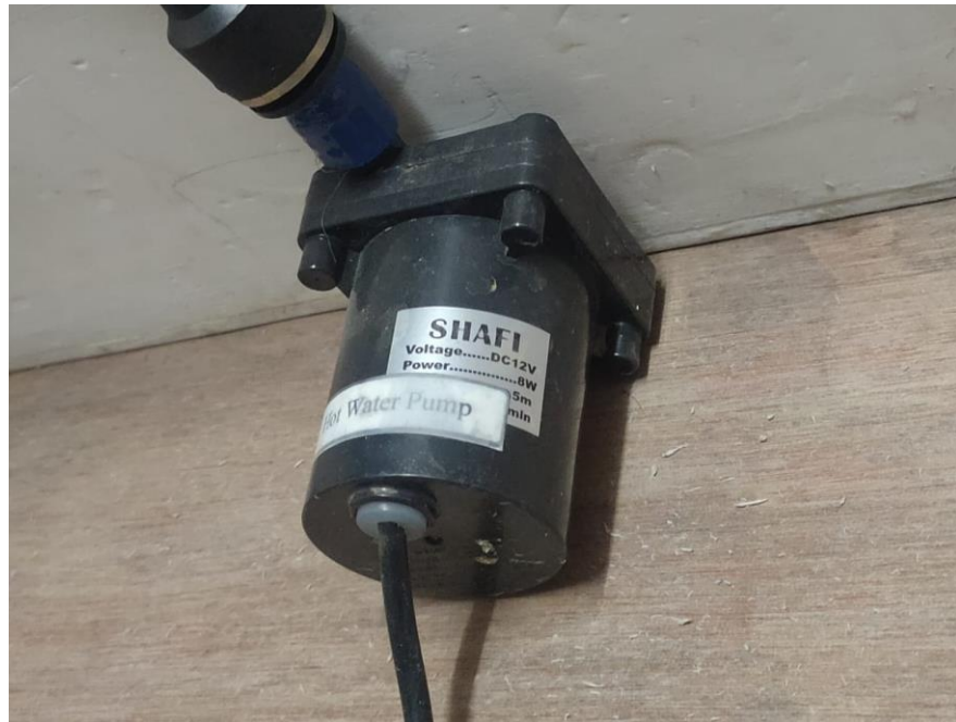
Fig. 3.8: Centrifugal water Pump.
