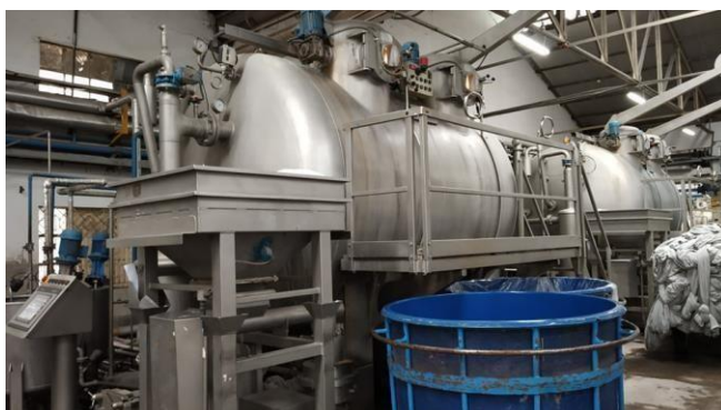
Fig. 3.23 Athena HTHP dyeing machine
