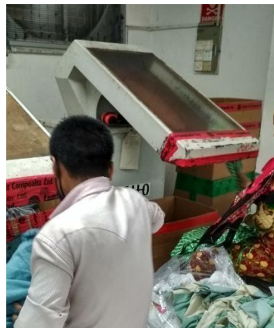
Fig. 3.11 NISHO thread sucking machine
