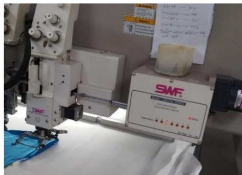
Fig. 3.12 Automatic multi-head Tapping embroidery machine
