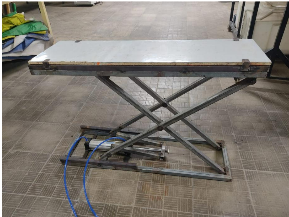
Fig 3.8: Frame of Pneumatic Lifting Table
