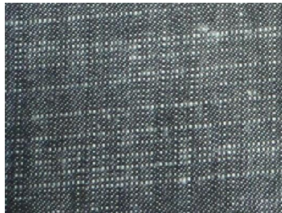
Figure 23: Fabric with skew
