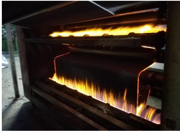
Figure 20: Singeing process in ADML
