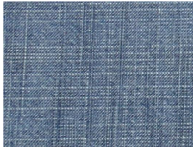
Figure 24: Fabric without skew
