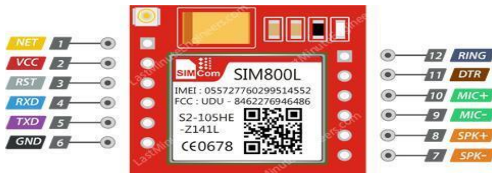
Figure 3.11: GSM Module Pinout
