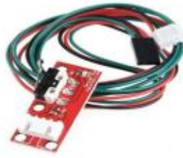
Figure (3.12): End stop switch
