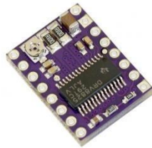
Figure (3.4): Dvr8824 Stepper motor Drivers with heat sink
