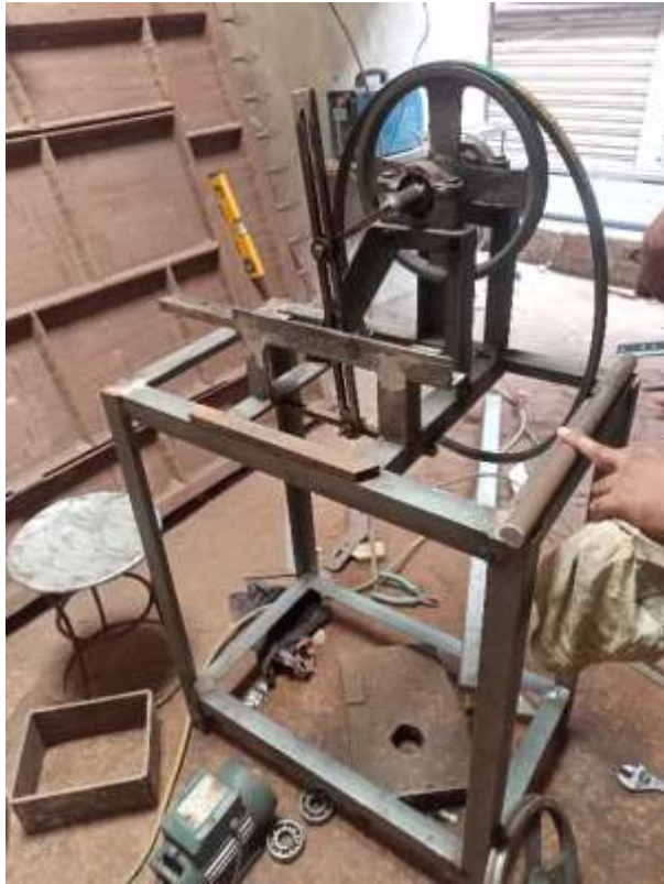
Fig 21: Construction of shaper Machine
