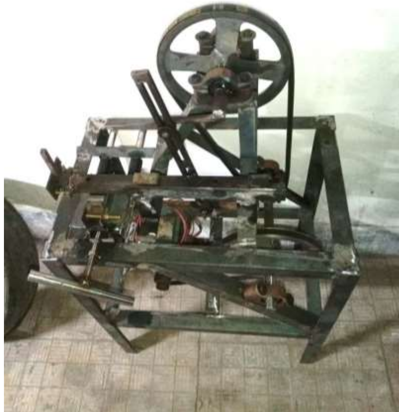
Fig 12: Crank And Slotted Link Mechanism
