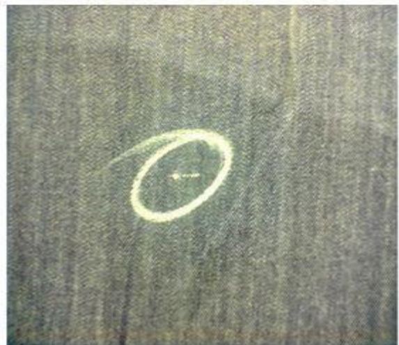
Figure: Faulty Slub
