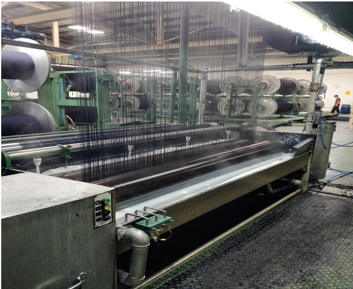
Figure 6.4: Yarn passing through size bath
