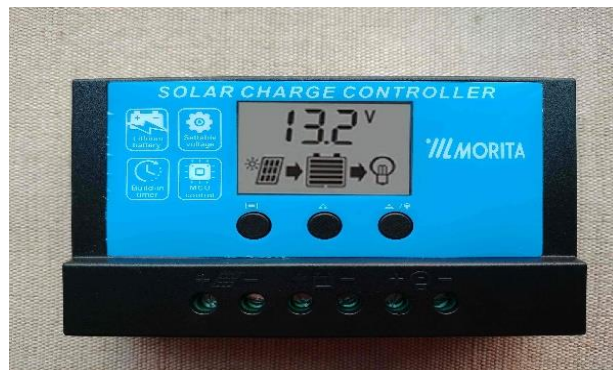
Fig-2.14: Charge Controller
