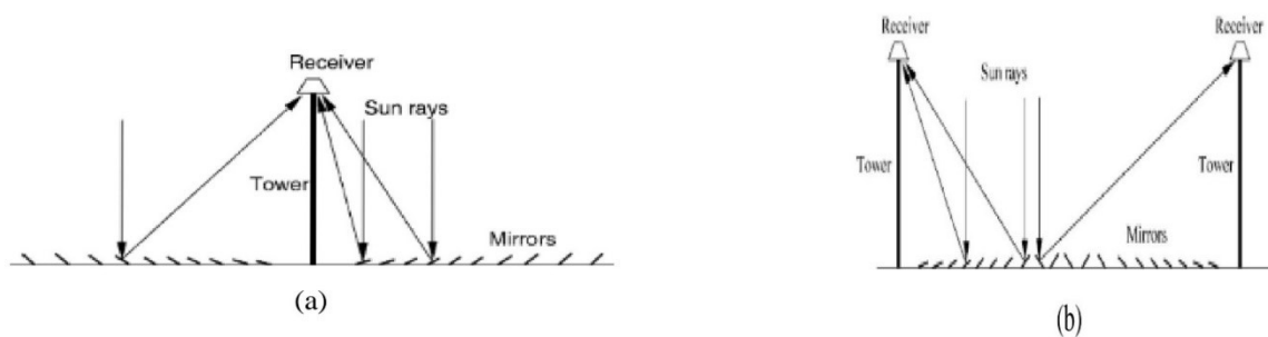
Figure No 3. 5: (a) Linear Fresnel Reflector, (b) Compact Linear Fresnel Reflector (Kalogirou,2004)
