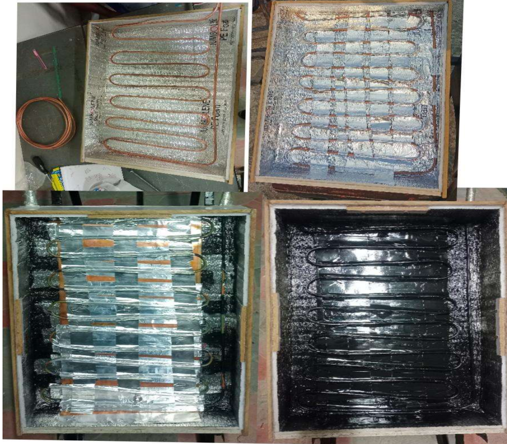
Figure No 4. 2: Steps of the Construction of FPSC
