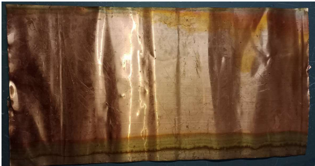
Figure No 4. 3: Copper Sheet Absorber
