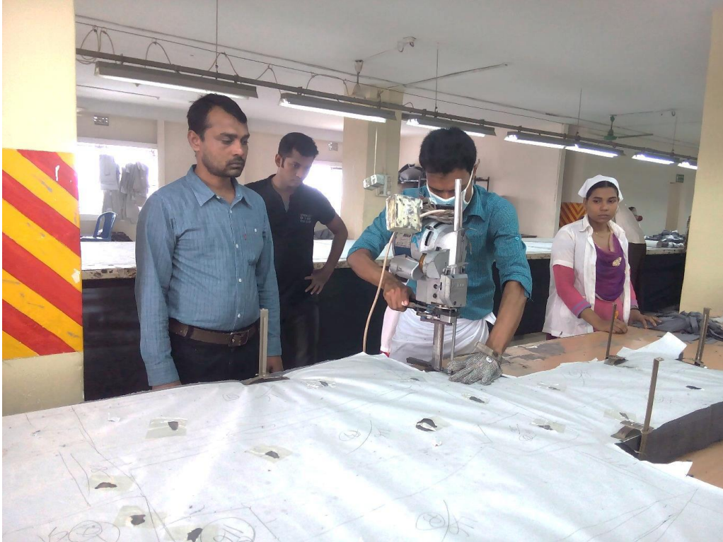
Figure -3.3: A worker is busy with cutting fabric layer
