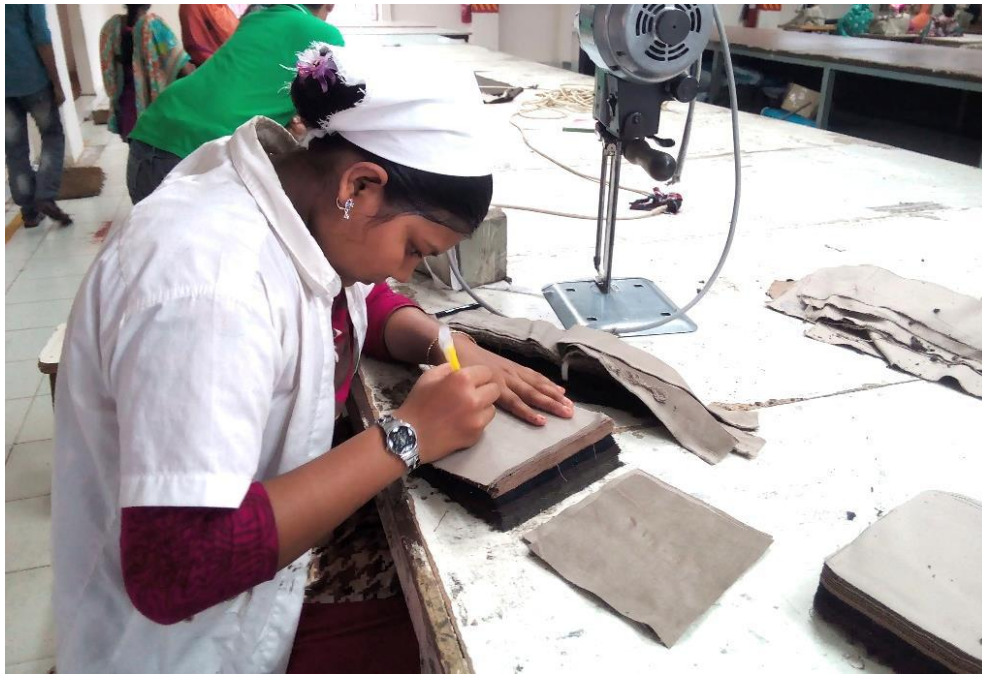
Figure-3.5: Fabric cut pieces are marked for shade variation and fastness test
