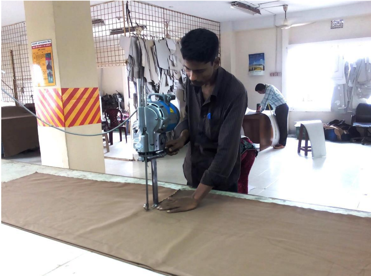
Figure-3.8: A worker is busy in test cutting of fabric
