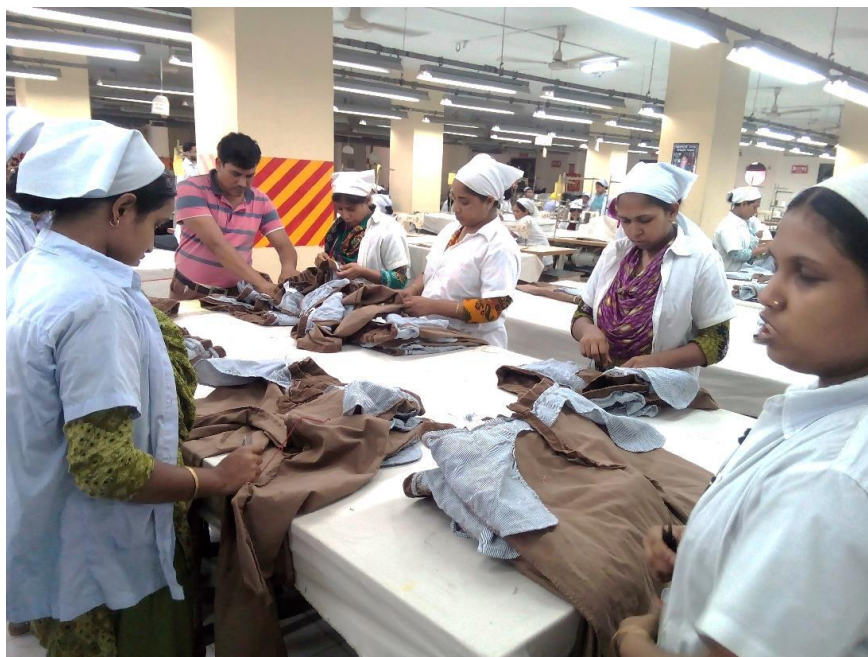
Figure-3.17: Workers are trimming the excess treads
