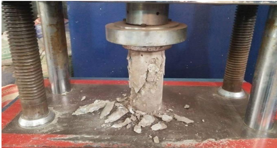
Figure 3.4: Compressive strength test of Cylinder
