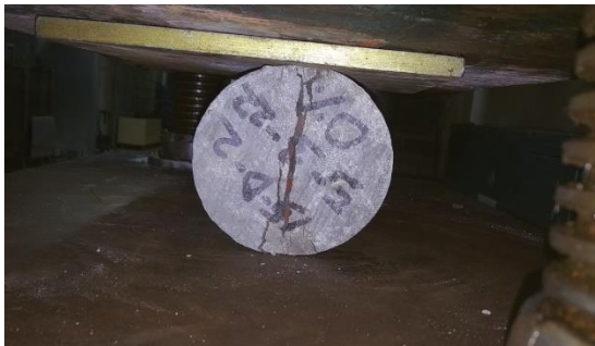
Fig. 4.6: Tensile Strength for 28 days.
