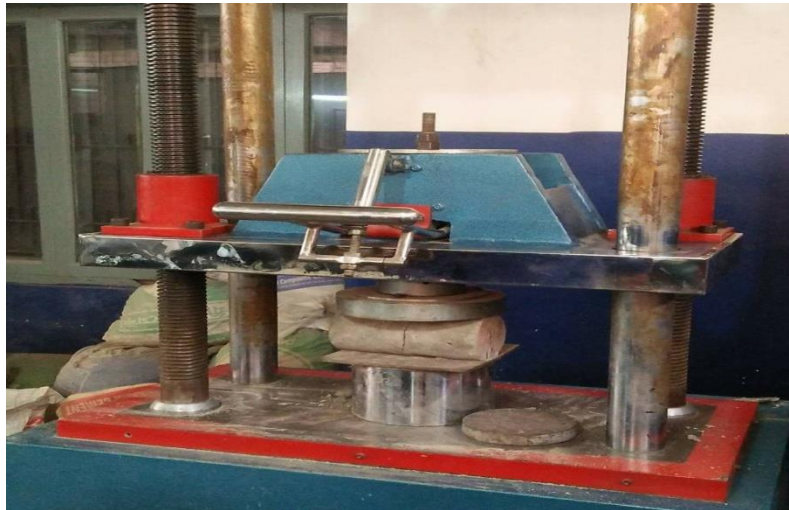
Figure 3.5: Splitting tensile strength test of cylinder
