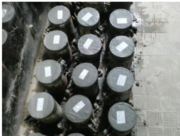
Figure 3.3: Molding of concrete specimens
