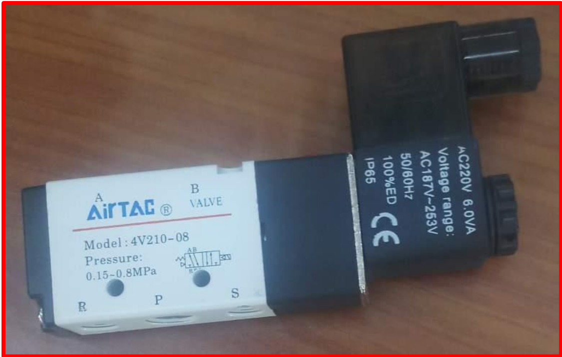
Figure 3.6 Piloted Type Electrical Solenoid 5 way, 2 positions Valve
