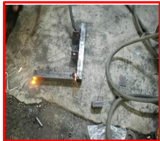
Figure 4.1 Cutting Operation of MS Plate
