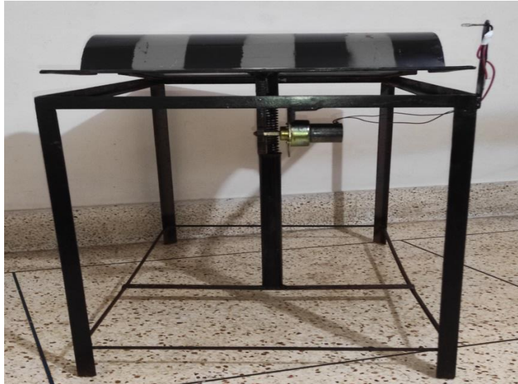
Figure 1.1: Electricity Generation by using Speed Breaker
