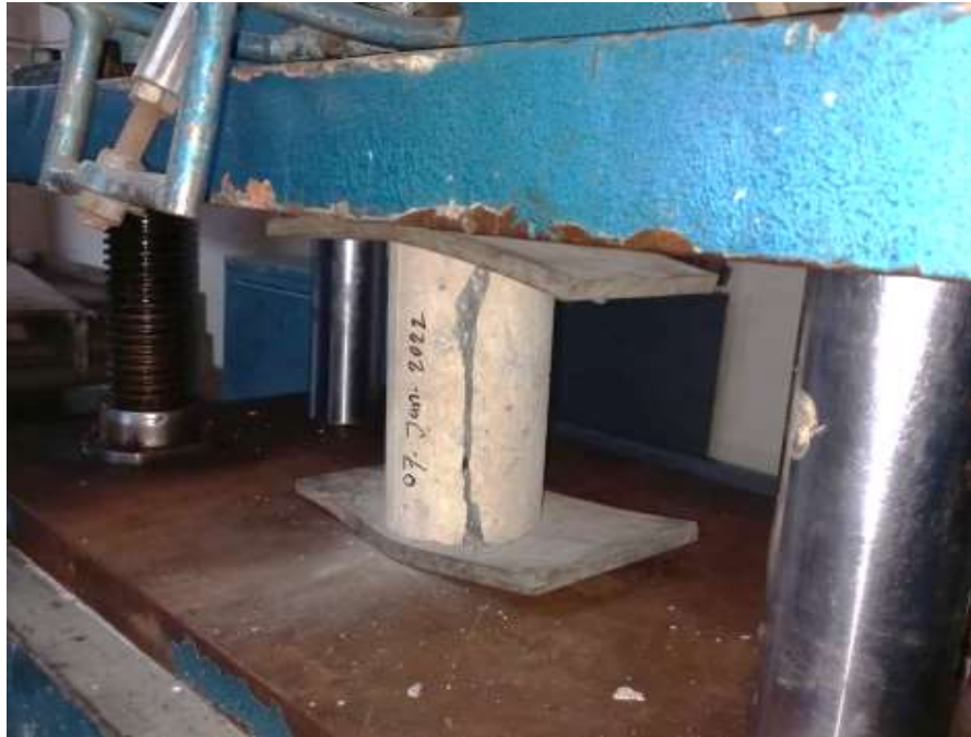
Fig 4.1: Compressive strength test of Cylinder No-1 of Batch Plant concrete.
