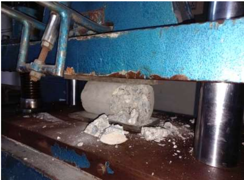
Fig. 4.4: Crashed concrete of Cylinder No-3 of Batch Plant concrete.
