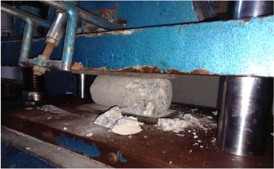
Fig:3.11: Tensile strength test of concrete by Universal Testing Machine (UTM).
