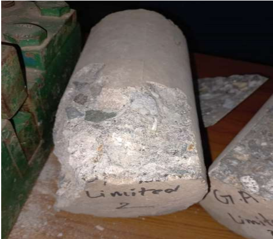
Fig. 4.3: Crashed concrete of Cylinder No-2 of Batch Plant concrete.
