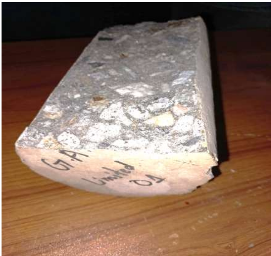
Fig. 4.2: Crushed Concrete of Cylinder No-1 of Batch Plant concrete.
