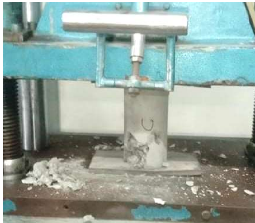
Fig. 4.6: Compressive strength test of Cylinder No-3 of Ready-mixed concrete.
