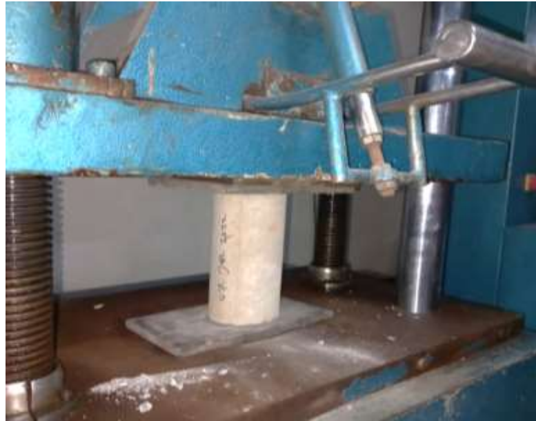
Fig:3.10: Compressive strength test of concrete by Universal Testing Machine (UTM).
