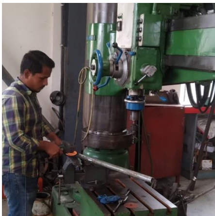
Fig: Drill machine operation
