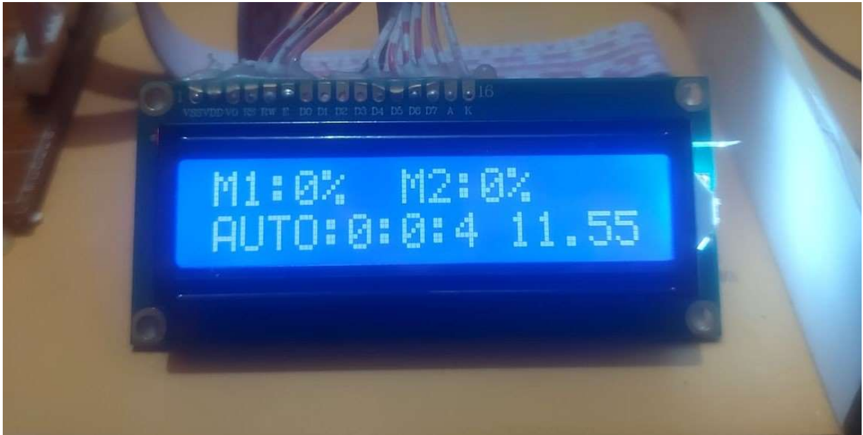
Figure 5.2: Showing the moisture level and pump status on LCD
