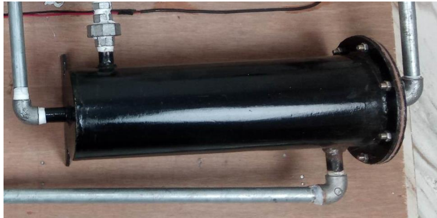
Figure 3.5: Gear Exchanger Tube
