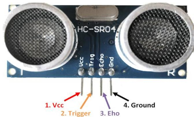
Figure 3.24: Ultrasonic Sensor Pin Out
